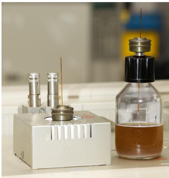
Fig. 2.3: SEP (with PDMS-sleeved stalk) installed in a sample bottle containing caracal urine and in a GC injector at 230 °C.
