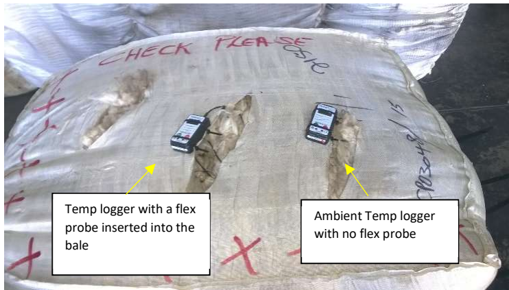
Figure 3 : Temp loggers mounted on a bale (pressed bale loosened). Flex probe was inserted to the middle of the bale.
