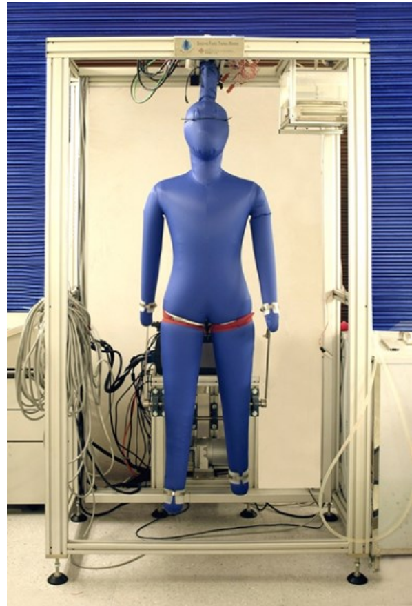
FIGURE 1: WALTER™ THE FABRIC SWEATING MANIKIN (SOURCE: FAN, NO DATE)
