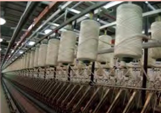
Spinning twists the fibres into a continuous yarn
